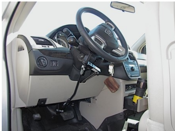
Hand Controls for Car. Note Rotated Seat-Back. This Allows Warren to Transfer from His Wheelchair to the Driver's Seat.
