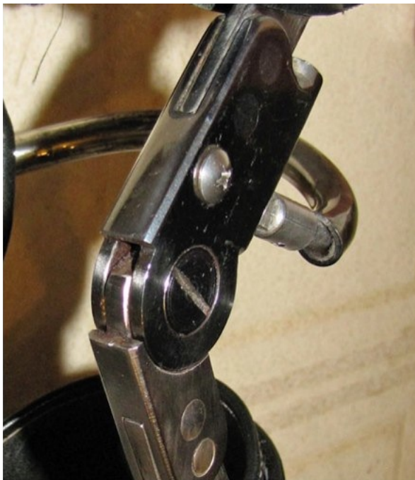
Locking Mechanism with Tygon Sleeve
