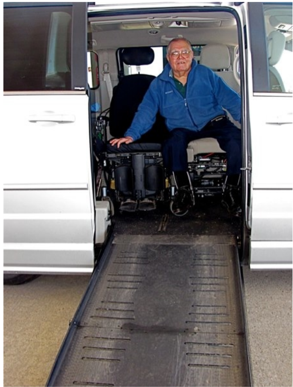
Warren on Driver’s Seat in the Van. The Seat is Rotated and Moved Back so that He Can Transfer to His Wheelchair. The Seat Will Be Moved Forward and Warren Will Exit on the Ramp on the Side of the Minivan. Note the Far Forward Position of the Passenger Seat. With Wheelchair and Minivan, Warren Has Independent Mobility.
