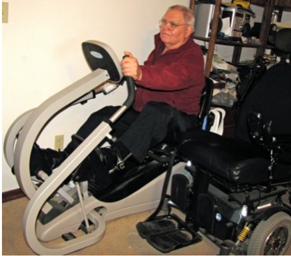
Warren Exercising with the NuStep. His Feet Are Strapped to the Pedals. The Handles Are Hard-Coupled to the Pedals so that Warren's Legs Are Moved as His Arms Move.
